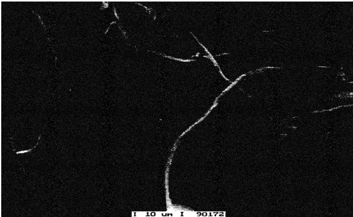
PLATE 11 Example of CI fiber. Note the variation in fiber diameter.
