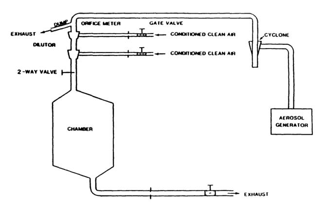
FIGURE K3 Schematic of the Nickel Subsulfide Aerosol Delivery System
