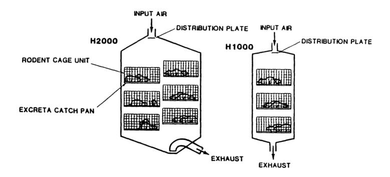
FIGURE K4 Schematic of the H1000 and H2000 Exposure Chambers
