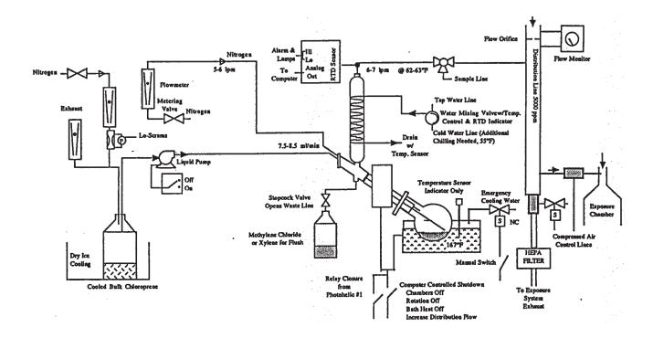
FIGURE K3 Schematic of Generation and Delivery System for the 16-Day Studies
