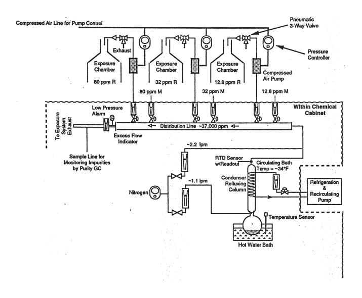
FIGURE K5 Schematic of Generation and Delivery System for the 2-Year Studies
