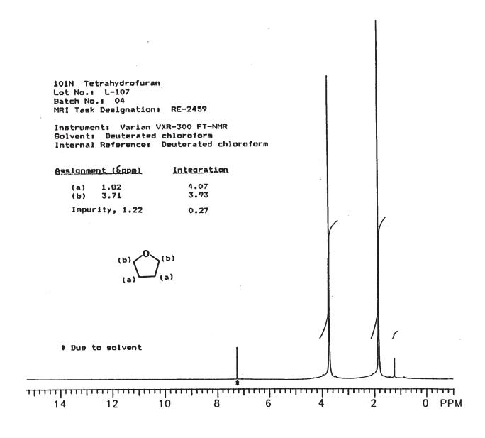
FIGURE H2 Nuclear Magnetic Resonance Spectrum of Tetrahydrofuran
