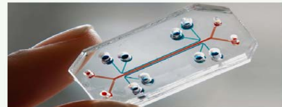
Figure 5. Lung-on-a-chip used to mimic pulmonary edema (Image Source: The Wyss Institute for Biologically Inspired Engineering)
