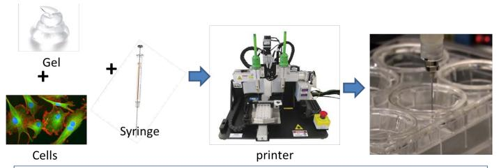
Hydrogel polymer is mixed with cells and loaded into syringe. The printer "3D prints" the cell/gel mixture in a layer by layer approach.
