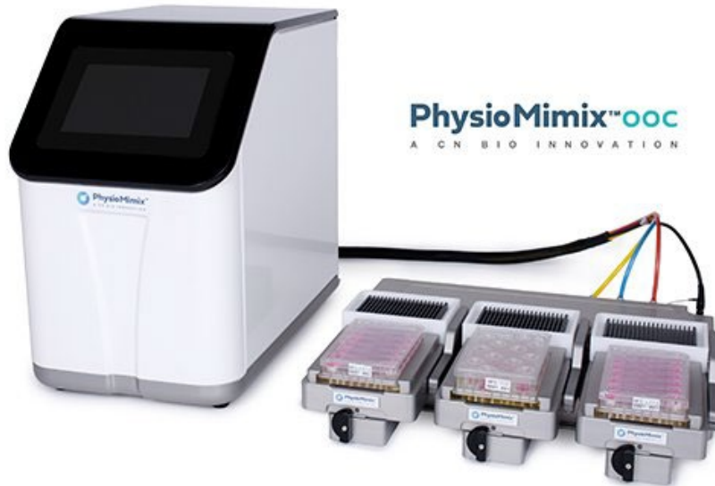
Figure 14. The PhysioMimix OOC microphysiological system. The controller supplies the pneumatic pressure and acts as a center for commands. The dock is where the system sits inside the incubator, delivering the pneumatic pressure. The drivers and plates are the mobile parts of the system where the cell culture takes place. Taken from CN-Bio IFU PhysioMimix System 000264
