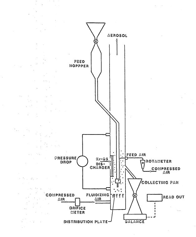
FIGURE I2 Fluid Bed Generator
