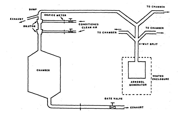
FIGURE I3 Aerosol Dilution/Delivery System
