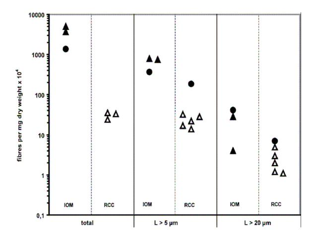
Figure 4-4. Concentration of fibers in lung tissue vs. size categories of fibers from rat inhalation studies conducted at two different laboratories
