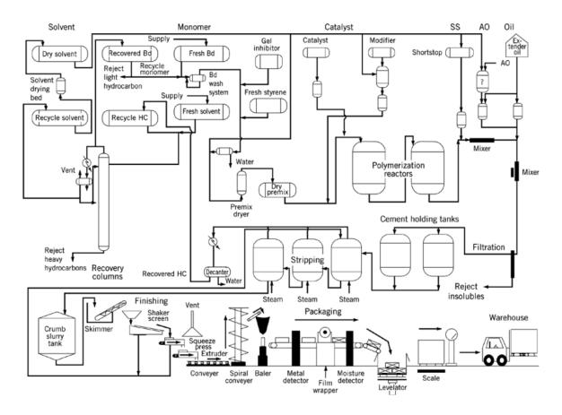
Figure 2-8. Solution styrene-butadiene rubber manufacture by continuous process Bd=butadiene, HC=hydrocarbon, AO=antioxidant, and SS=shortstop.
