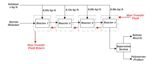
Figure 2-9. Polymerization of polystyrene by the continuous process Source: Cheresources 2008a.
