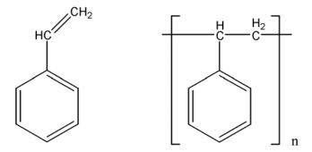
Figure 1-1. Chemical structures of styrene and polystyrene
