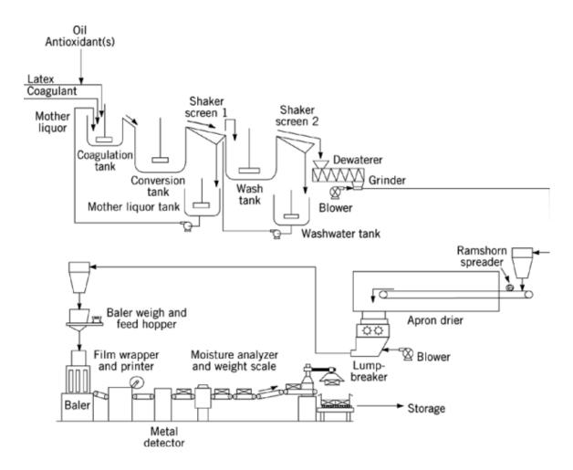
Figure 2-7. Typical emulsion styrene-butadiene rubber finishing process Source: Lattime 2000
