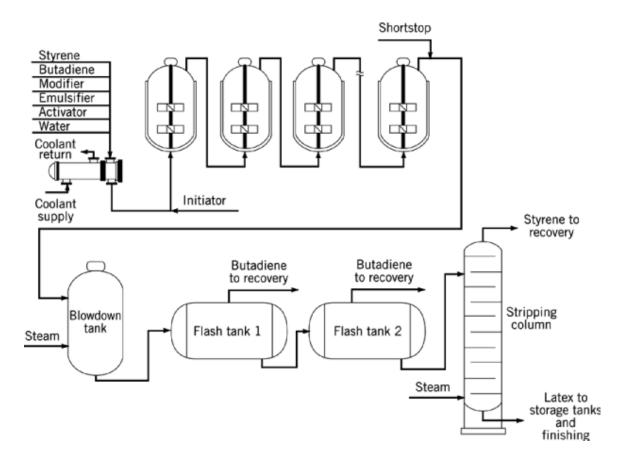
Figure 2-6. Typical continuous emulsion styrene-butadiene rubber polymerization process
