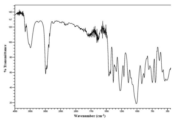
Figure A-1. Infrared Absorption Spectrum of Tris(chloropropyl) Phosphate (Lot M072911NP)
