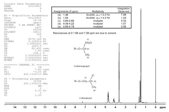
Figure A-2. <sup>1</sup>H Nuclear Magnetic Resonance Spectrum of Tris(chloropropyl) Phosphate (Lot M072911NP)
