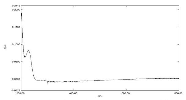
Figure A-4. Ultraviolet/Visible Spectrum of Tris(chloropropyl) Phosphate (Lot M072911NP)
