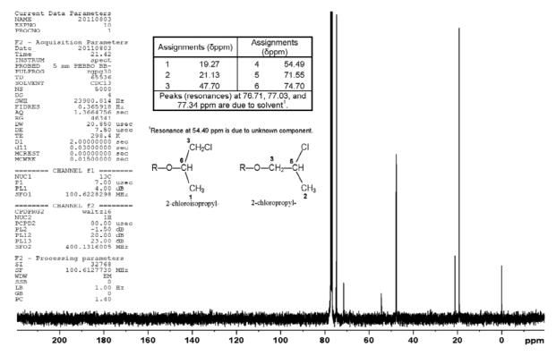
Figure A-3. <sup>13</sup>C Nuclear Magnetic Resonance Spectrum of Tris(chloropropyl) Phosphate (Lot M072911NP)
