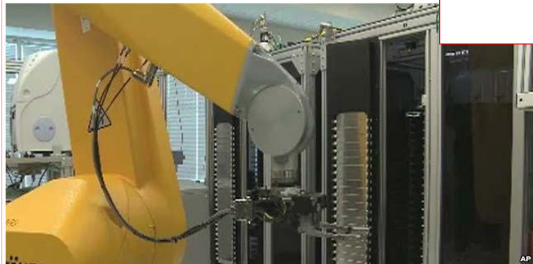
This high-speed robotic tester is revolutionizing routine chemical toxicity studies by screening thousands of chemicals each week for potential human toxicity
