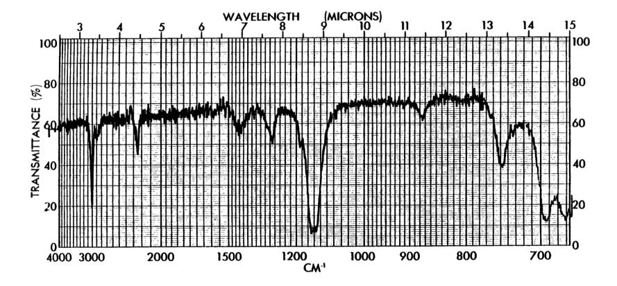
FIGURE 1. INFRARED ABSORPTION SPECTRUM OF TRIBROMOMETHANE (LOT NO. 71221)
