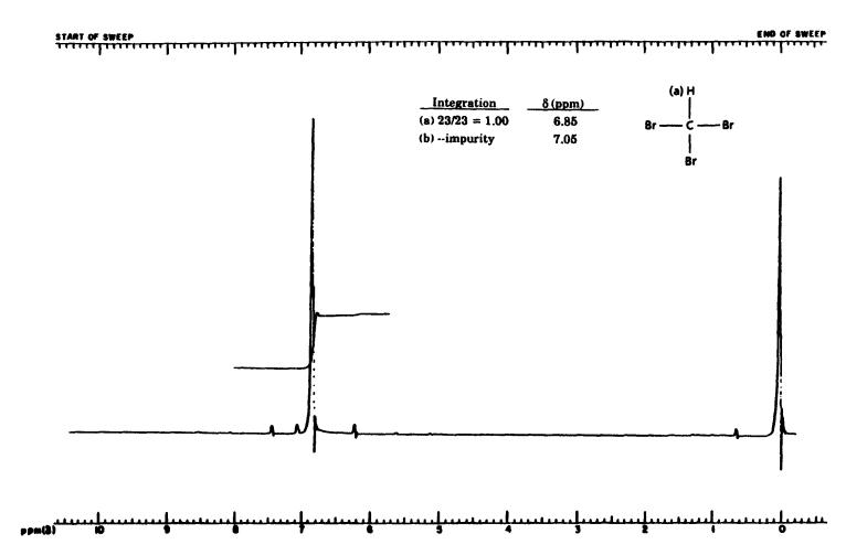
FIGURE 2. NUCLEAR MAGNETIC RESONANCE SPECTRUM OF TRIBROMOMETHANE (LOT NO. 71221)
