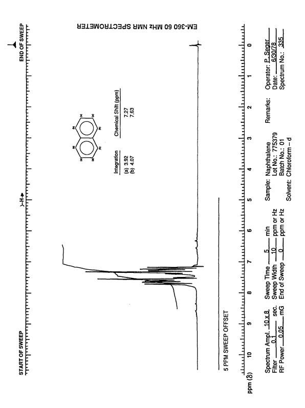
FIGURE E2 Nuclear Magnetic Resonance Spectrum of Naphthalene
